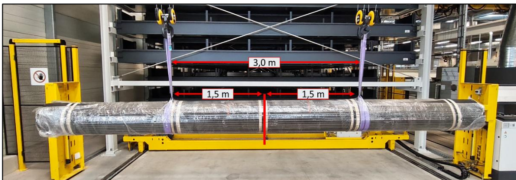
Figure 9: Positioning of the round slings under the pipe bundle
